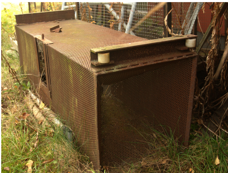
Fig. 16. A metallic box used for lamprey catching at the hydroelectric power plant dam in the River Ljusnan, in Sweden. Most of the lampreys are transported and released upstream of the dam. 14 October 2011. Photo: Kjell Sjöberg.
