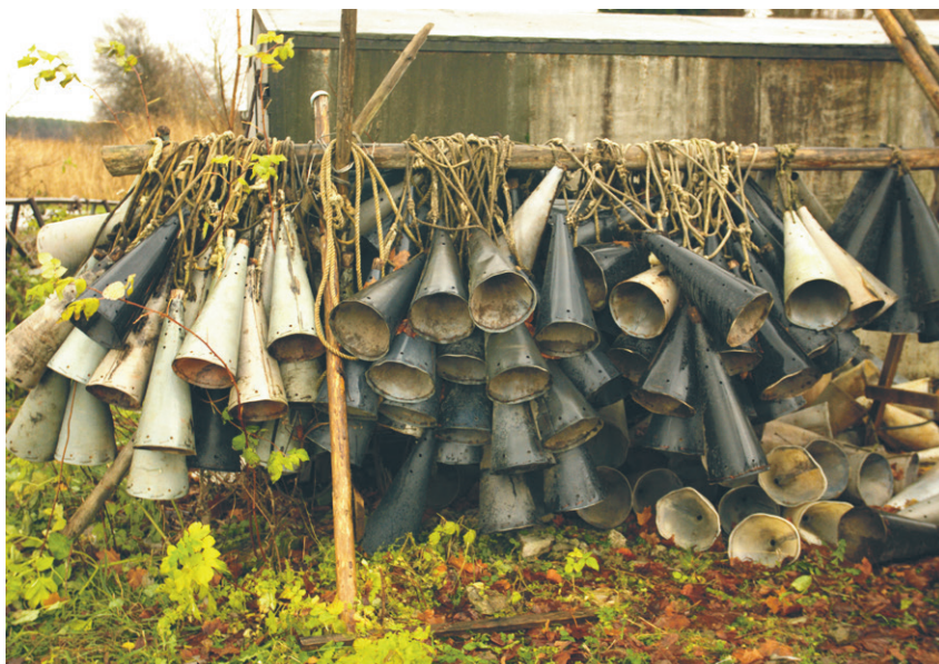
Fig. 89. Cone gear at the River Narva, Estonia. About 50 cones are attached less than one metre apart from each other along a rope. 7 November 2012. Photo: Kjell Sjöberg.
