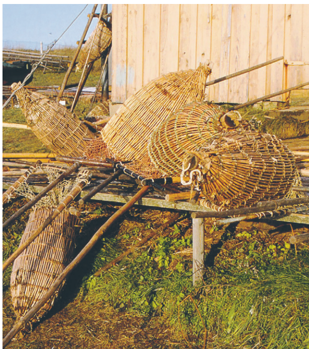
Fig. 64. Gear constructed as a combination of baskets and mesh. The gear is emptied in the end of the trap, which during fishing position is closed with a wooden tap. Although the water flow was pressing against the wooden trap from inside, the tap was only very rarely flushed out of the gear, so there was no specific arrangement for keeping the tap in place. 18 The River Salaca 1992. Photo: Kjell Sjöberg.
