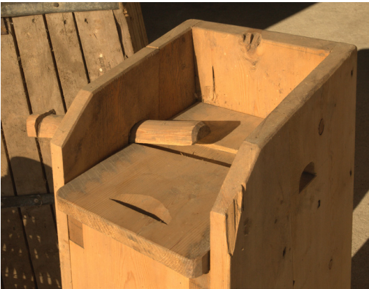
Fig. 11b. Sliding stopper and its locking wedge (Swedish stängningslucka med lås ) on a wooden log from the River Umeälven owned by Rickard Danielsson at Klabböle. There is a groove in the sliding stopper where the pin acting as a locking wedge is slid into position. In that way it prevents the stopper from moving in either direction. 18 March 2013. Photo: Kjell Sjöberg.
